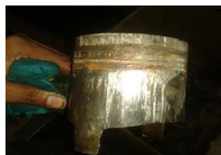
Fig.5. Worn out piston due to overheating
