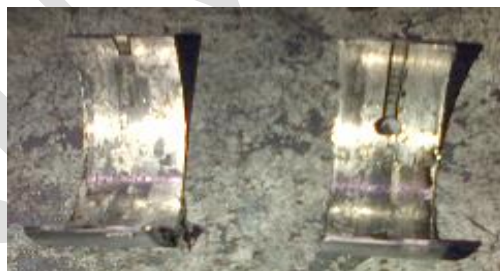
Fig.4. Scratches on upper main bearing caps
