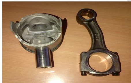
Fig.10. Hydrostatic Lock Effect
