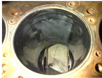
Fig.7. Worn out cylinder surface
