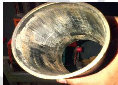
Fig.8. Worn out piston sleeves due to of badly overheated piston
