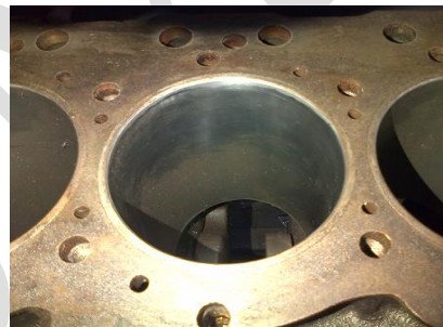
Fig.11. Cylinder in good condition
