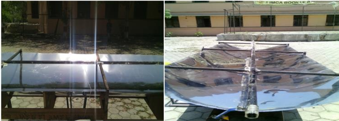
Figure : Experimental setup of solar parabolic trough
